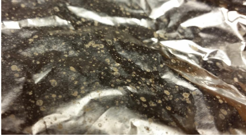
Figure 27: Electrospinning PS: D-limonene solution with 20% PS at 28 kV
