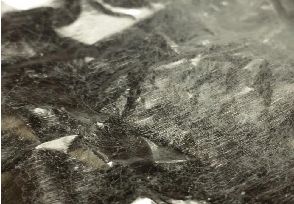
Figure 24: Nanofiber mesh - PS: toluene solution with 10% PS.
