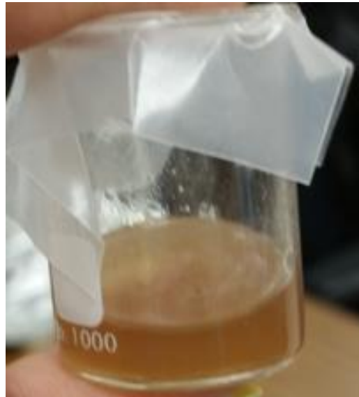
Figure 5: Homogenous CoO-ATO PS: toluene solution after 10 minutes of stirring
