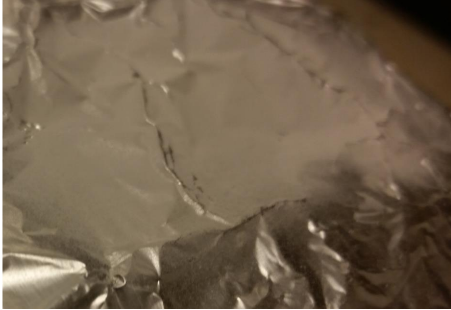
Figure 25: Nanofiber mesh - PS: toluene solution with 20% PS.
